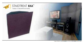
The STAIDTREAT BXA" is a low-frequency absorption panel. It is tuned to 63 Hz and is meant to be placed in 90° corners. The principle used to develop the STAIDTREAT BXA\* is exclusive to JOCAVI®. It combines an HIPS box, which has two appropriately enhanced closed resonance chambers inside, with mass and density components. These components have been specifically developed for this model.
