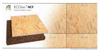
ECOiso "NCF" is a sound insulation material composed by one sheet of Cork Agglomerate and one board of high-density recycled wood fibers. This material was thought in order to reduce transmission of sound and vibration in the floors of residential and commercial buildings. It can also be used on walls and ceirings.
