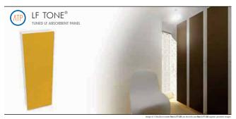
The LF TONE\* is a low-frequency membrane absorbent panel to be used on walls or ceilings. It was conceived as a whole box and with a membrane designed to provide more sensitivity to the low pressure sound waves. It is tuned to 250Hz and it also has an effective performance at lower frequencies.
