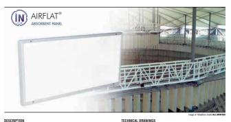
The AIRFLAT\* is an additional option as an absorption panel. This panel's structure is made on an aluminum frame, which gives the product a good robustness; the absorbent layer is built in a mineral fiber plate with viselike fabric that makes the finishing.
